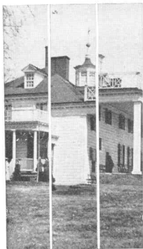
As image will appear when Range Finder is racked too far forward.
