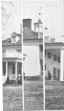
As image will appear when Range Finder is racked too far back.
